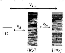
Fig. 1. Energy level scheme for the model studied. The initial level (s) is coupled to the continua (or quasicontinua)  $\{|I\rangle\}$  and  $\{|m\rangle\}$  (also denoted L and M in the text). In the constant coupling model (CCM)  $V_{Sl}$ ,  $V_{ml}$  and  $V_{Sm}$  are taken to be independent of the level indices I and m. In the random coupling model (RCM) they are taken as random functions of these indices.
