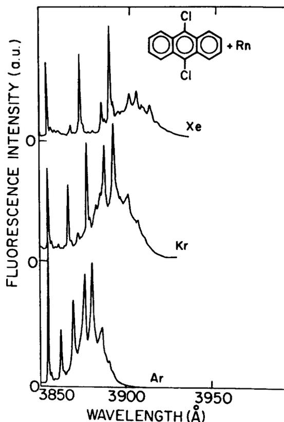
FIG. 3. Rare-gas complexes of 9, 10-DCA. The nozzle diameter was  $20\ \mu$  and its temperature was  $170\ ^\circ\text{C}$ . The argon, krypton and xenon backing pressures were 800, 600, and 300 Torr respectively.
