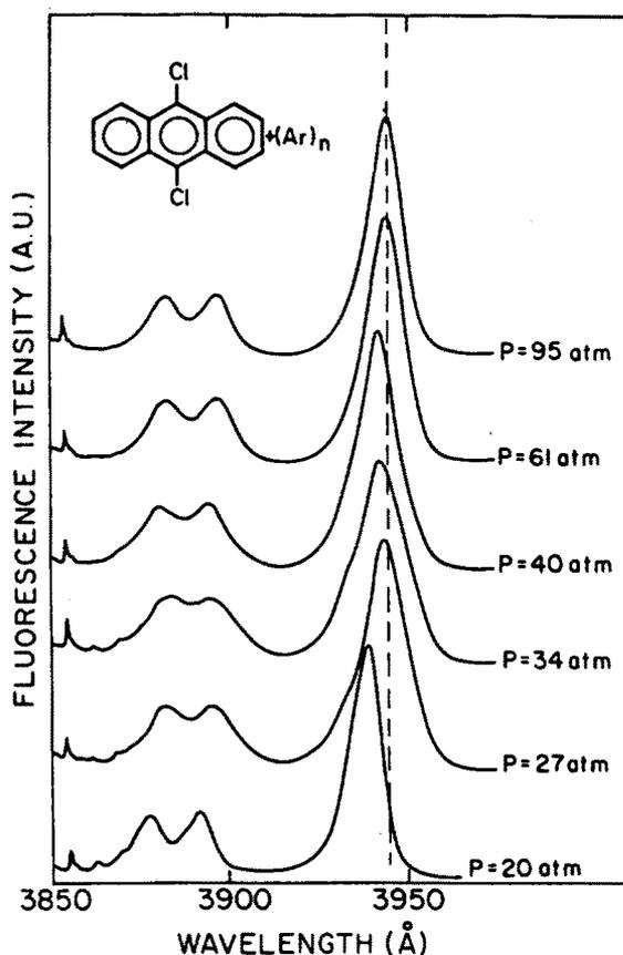
FIG. 9. Spectral manifestation of a structural change in 9, 10-DCA clusters with argon. The excitation spectra are plotted at the various indicated argon backing pressures. The dotted line is drawn to emphasize the slight blue shift at around 40 atm. 20  $\mu$  nozzle diameter was used at 190 °C.
