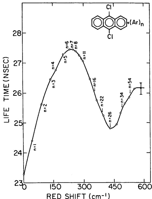
FIG. 7. The emission lifetime of argon complexes of 9, 10-DCA vs their spectral red shift. The spectral positions of the first eleven clusters are indicated. In each case the lifetime measurement was performed using several nozzles and at argon backing pressure where the yield of that cluster was optimized.
