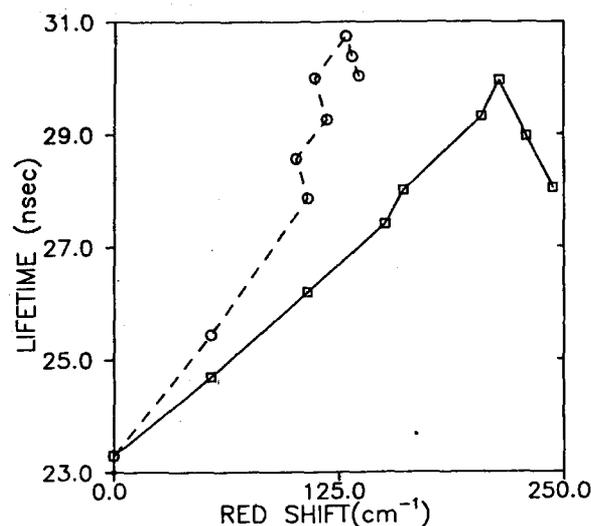
FIG. 11. Calculated radiative lifetime of several dichloroanthracene-Ar<sub>*n*</sub> ( $n = 0, \dots, 8$ ) complexes, plotted against the calculated frequency shifts. Circles connected by a dashed line are results of model (a) (see the text) while squares connected by a full line are results of model (b). See the text for the structures of the complexes.
