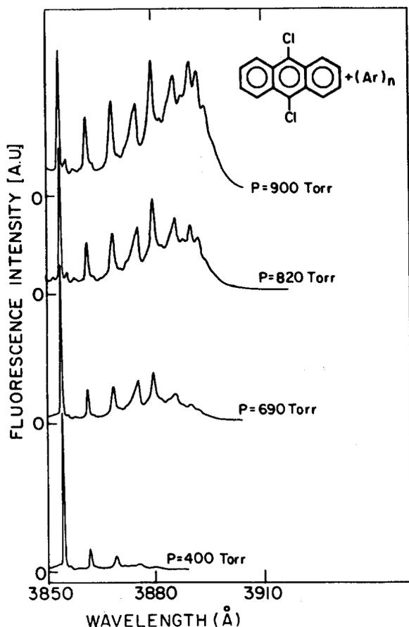
FIG. 2. The argon backing pressure effect on the generation of 9, 10-dichloroanthracene complexes with argon. The nozzle diameter was  $20\ \mu$  and its temperature was  $160\ ^\circ\text{C}$ .
