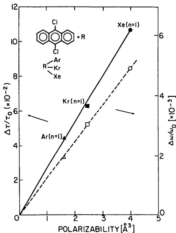
FIG. 4. The added pure radiative lifetime and the spectral red shift of argon, krypton, and xenon van der Waals complexes with 9, 10-dichloroanthracene against the rare-gas atom polarizabilities.
