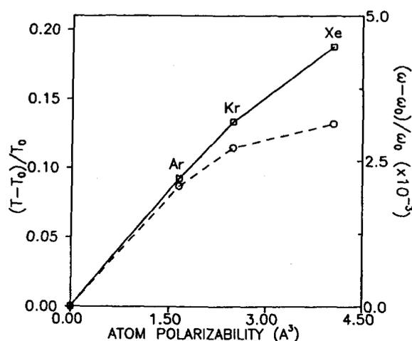
FIG. 12. Relative lifetime shifts (squares connected by a full line; right axis) and relative frequency shifts (circles connected by a dashed line; left axis) of DCA complexed with one Ar, Kr, or Xe atom, plotted against the atomic polarizability of the rare-gas atom. Model (a) for the molecular charge distribution was used in this calculation.
