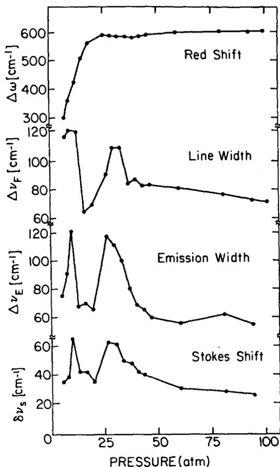
FIG. 10. The spectral red shift, excitation line width, emission line width and its Stokes shift of 9, 10-DCA clusters with argon against the nozzle backing pressure. Measurements are at the electronic origin as shown in Figs. 6 and 9. The nozzle diameter was  $20\ \mu$  and its temperature was  $190^\circ\text{C}$ .
