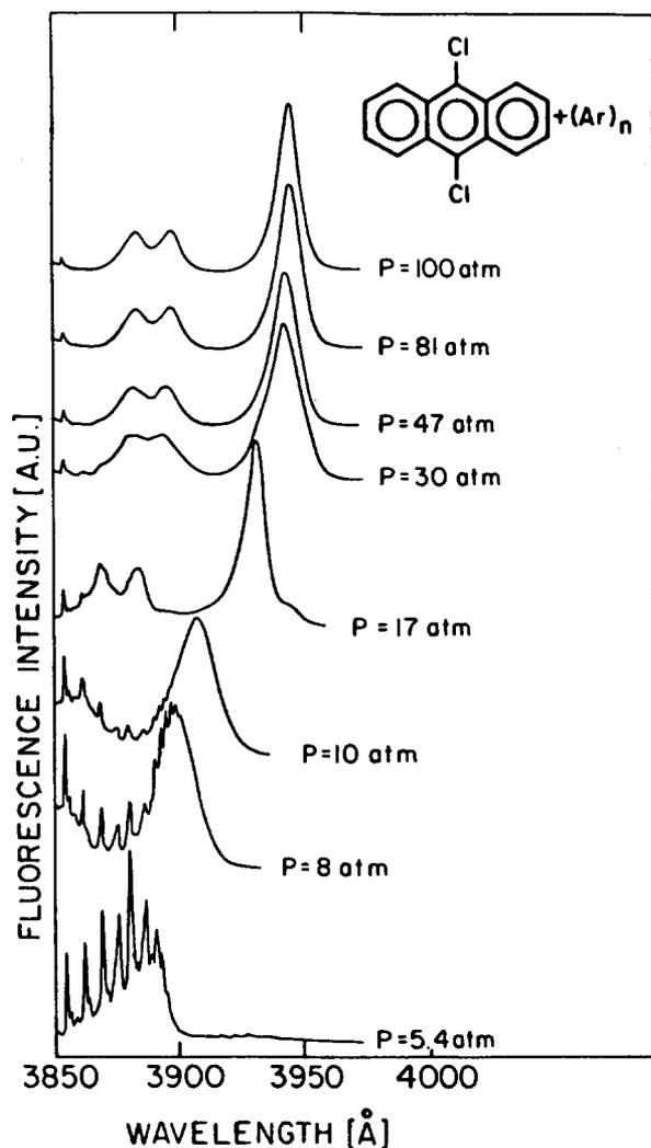
FIG. 6. The pressure effect on the spectroscopy of 9, 10-DCA clusters with argon. The nozzle diameter was  $20 \mu$  and its temperature was  $190^\circ\text{C}$ .
