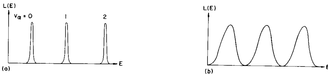
Fig. 2. Lineshapes of a large molecule with sequence congestion effects at a finite temperature. a) All frequencies equal in ground and excited states, b) a real life situation. Frequencies in excited state are lower than in ground state.
